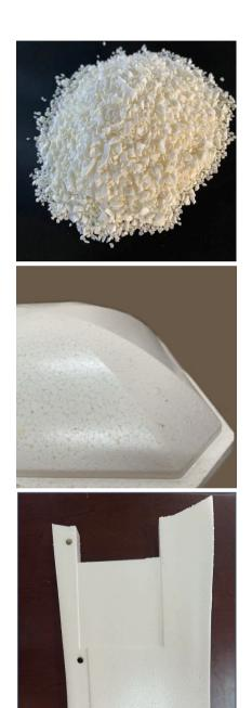
ARCHCELL® FIT is a type of PMI granule that can be foamed directly in the mold by heating to form a specific shape, which has obvious advantages in the molding of complex shaped components. It is available in two forms: one is a copolymer granule; the other is a granule that has been pre-foamed at a specific temperature and time.
